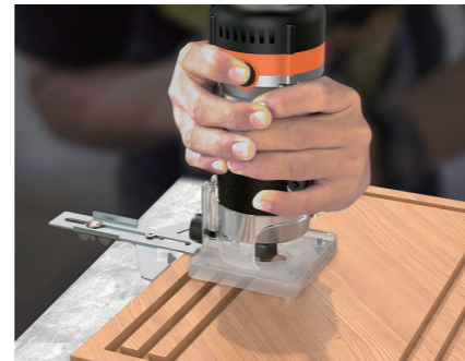
Fix with a baffle on one side to ensure that the milling groove position is not offset, and hold tightly with both hands to push the milling groove machine
