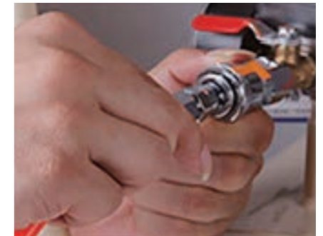
After inflation is complete, connect one end of the hose to the air pump and the other end to the air gun
