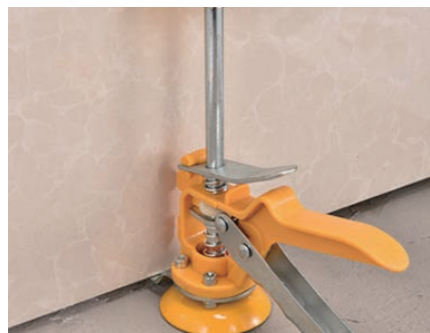
Insert the top lifter into the bottom of the board
