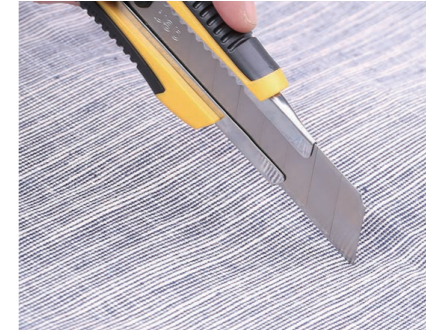
When the blade is not sharp, the blade can be crushed and then extended
