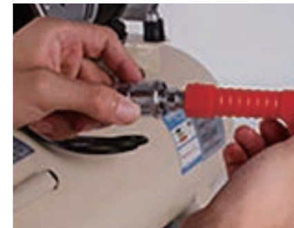
Connect air pump and steel nail gun
