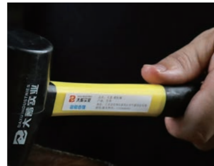
Grasp the end of the handle tightly, apply force evenly, and pay attention to hand protection
