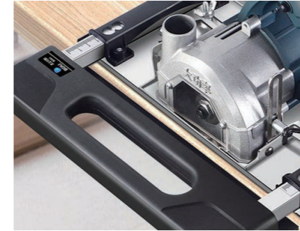
Press against one end of the wall panel, confirm the cutting position, and fix the cutting machine
