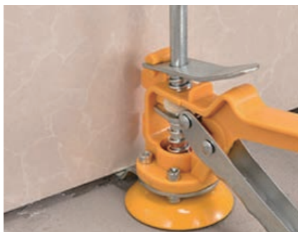
Push the handle up to lift the wall panel, and wait for it to be fixed before removing it
