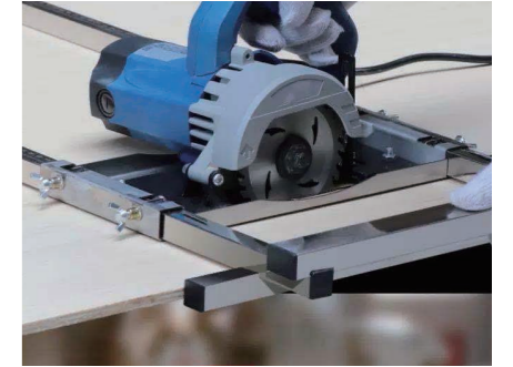
Gently push the cutting machine with uniform force and speed, pay attention to hand safety
