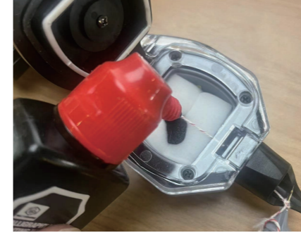
Open the ink cartridge and put in an appropriate amount of ink
