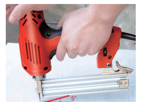
To avoid the steel nails from not being inserted firmly,use your hands to firmly press down on the base
