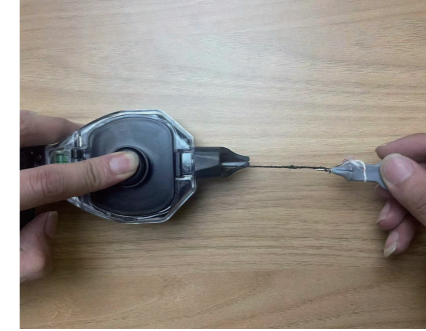
Hold down the valve while pulling the line to allow the line to absorb ink
