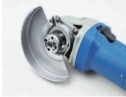
Turn off the fixing screw, insert a suitable cutting piece, and fix the screw
