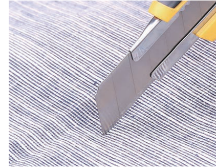
Install the blade so that it protrudes about 3cm
