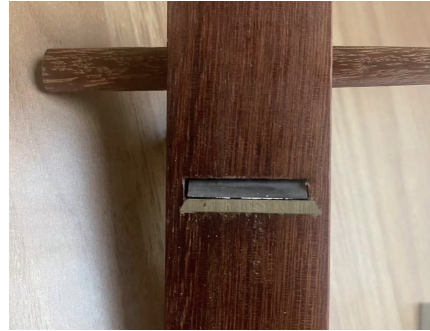
Adjust the blade to extend a little, basically level with the base
