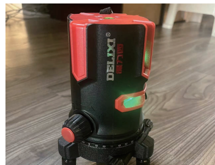
It needs to be placed flat and reach the level without any warning sound
