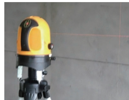
Adjust the height of the spirit level using a bracket according to the actual situation
