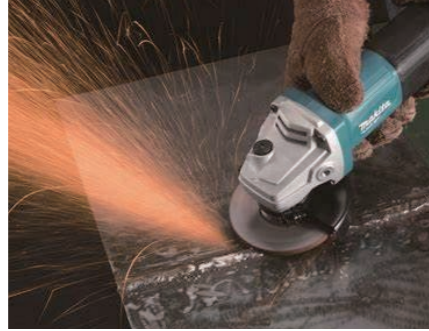
When starting the machine, it is necessary to hold it tightly with both hands to prevent vibration
