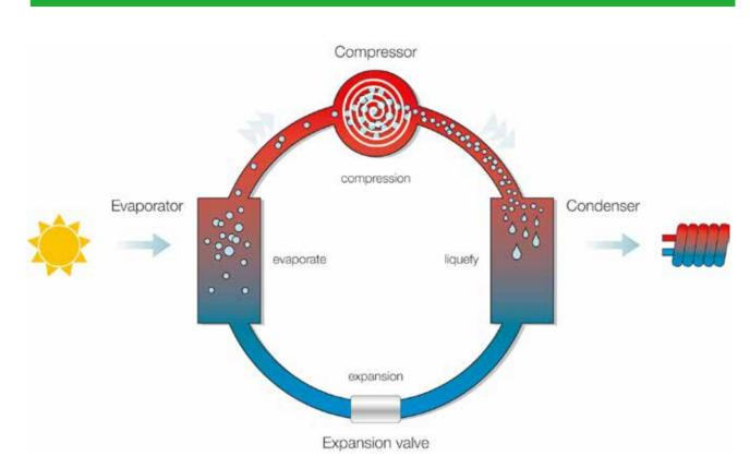
Heat pump water heater extracts energy from the air and uses it to heat water. It uses 1 time power to drive the compressor and brings 4.3 times heat to the water. this is what we called coefficient of performance(COP). With COP up to 4.3.
