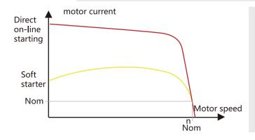
Soft starter for option, reduce the starting current and starting stress, extend the service life of the motor and related equipment. Smooth start and soft stop avoid the surge problem and water hammer effect of traditional starting equipment.
