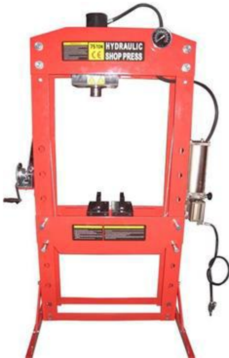
75TON SHOP PRESS PM1904B-- (LIGHT DUTY)
